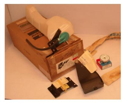
The E-Body has two bracket system with the first mounting directly to the side of the radiator support. The second is a small bracket that provides support to the bottom of the bottle. I am more of a B-Body guy so I am not sure of what years this was first available for the E-Body.
