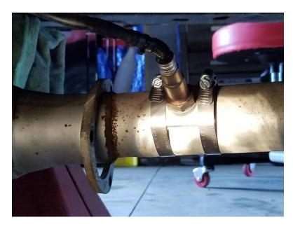
Next was getting the water temperature sensor installed. The easy way would have to have installed this in the water pump housing in the provided factory port. Again, we are talking about an old car and that plug was not coming out. I needed to improvise by adding a T to the hot water hose to install the sensor. It worked out in the end.
