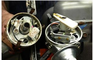
.Though all 1965-'67 A861 273 four-barrel engines got dual-point distributors, they were only installed on four-speed 340s in 1968-'71. For 1972, Chrysler's breaker-less electronic ignition was standardized on the 340 (optional in '71). Our 340 uses a Mopar Performance electronic unit (part No. P3690430, right). Total timing is set at 35 degrees BTDC
