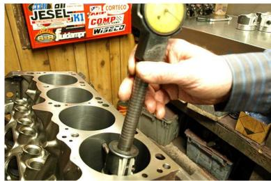
For our rebuild, the stock 4.04-inch bores were enlarged to 4.080 by a 0.040-inch cut on RAD's Rottler F79A boring machine. Torque plates were bolted to the decks before the Rottler HP6A diamond hone went to work. Sharing the same 3.312-inch stroke with the 273 and 318, the 340's extra cubes came strictly from its bigger 4.04-inch bores. Bore spacing is 4.46 inches
