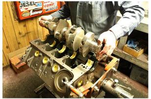
Some 11.6 pounds lighter than a forged 440 big-block crank, Donnie sets the crank in place. The cap bolts torque to 85 lb-ft in two steps. While 273 and 318 blocks have two core plugs per side, the 340
