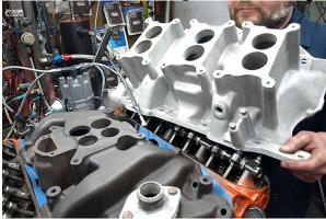
The stock dual-plane four-barrel manifold (46.6 pounds) is an excellent piece. The Edelbrock-sourced Six Pack (23.4 pounds) is the only aluminum intake manifold ever offered on the 340. A full two inches taller, the added runner and plenum volume are a huge bonus. Our Six Pack is a 1970 unit; Edelbrock still makes them
