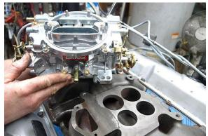
Lacking a vintage Carter AVS (1968-'70) or Thermo-Quad (1971-'73) we substituted an Edelbrock Performer 1405 for baseline testing. Its 600cfm rating puts it between the 570cfm AVS (1968-'70) and 750cfm TQ (1971-'73), both of which Chrysler claimed made the same 275 horsepower atop the 340
