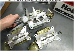
There's no Six Pack setup better than a brand new one, and Holley still sells 'em. Unlike swap meet stuff, no gurus have been inside tinkering, and the optimal factory settings are ready to deliver crisp cruising or neck-snapping, bog-free surges when wanted. The center carb (part No. 0-4792) has 1.50-inch diameter throttle blades and is rated at 350 cfm. The twin 500cfm outboard carbs (part No. 0-4790) are vacuum operated.
