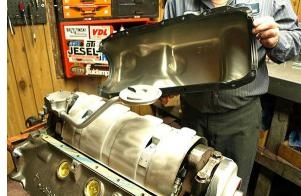
pickup tube and screen (part No. 72-S2) are from Melling. The stock pan was dented and rusty so a new 5-quart unit from Spectra (part No. CRB-09B) went on.
