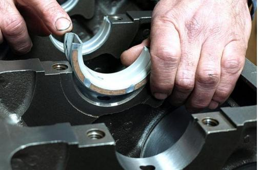
With the main saddles aligned on RAD's Sunnen align hone machine, the Clevite main bearings (PN MS963-P) are installed. The 340 block has thicker bulkheads and wall sections than the 318. Hemi legend Tom Hoover played a key role in developing the A105 340. Read Willem Weertman's book Chrysler Engines 1922-1998 (SAE Books) for the full story.
