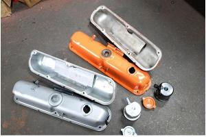
Gb Auto Metal Direct (AMD) supplied fresh 1970-spec 340 valve covers (part No. EF-3882AR), breather (part No. EF-3881-BTB1), and oil fill cap (part No. EF-3881-CAP). The original parts (in orange) can trap residual grime that can never be fully eradicated. AMD offers year-correct valve covers for all popular small- and big-block applications, not to mention a growing line of excellent, high-precision body panels.
