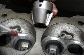
A "bowl hog" cutter (center) was inserted in the Rottler SGF8 seat machine to lightly dress the throats (left). We argued against this step to keep things stock for testing but were overruled by the engine owner. It's doubtful this work added more than a few clicks to the results with the mild cam. No other porting or hand blending was performed.
