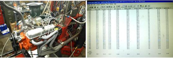
With the simple addition of 1 7/8-inch headers, output jumped to 352.1 horsepower at 5,300 rpm and 395.9 lb-ft of torque. In a 3,200-pound A-Body with 3.91 gears and traction, mid-thirteen second e.t.s are guaranteed.
