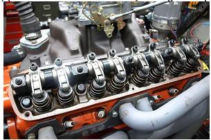
The roller rocker arm kit rendered the Chrysler's 7.500-inch 340 push rods too long for the job. Donnie found some 7.266-inch long, 5/16-inch diameter COMP Cams push rods (part No. 7809-16) from a Brand X application. The lifter preload was set at ½ turn beyond zero lash.
