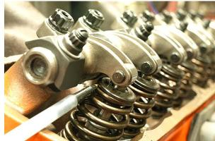
COMP Cams beehive valve springs (part No. 26986-16) and matching 1.340-inch diameter retainers (part No. 795-16) saved the day. The 10-degree locks were transferred and reused. With 123 pounds on the seat and 284 pounds at 0.500-inch lift, the tapered springs restored the ability to use the roller rocker kit. The pen points to the resulting clearance. Stock 340 valve springs were rated at 96/242
