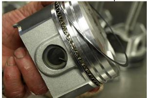
Hastings moly-faced rings (part No. 2M694-040) share the same 5/64, 5/65, 3/16 width as stock, and are gapped at 0.018 inch. The Sealed Power pistons feature anti-scuff coating on the skirts and deliver the same 10.5:1 compression as stock. Note the floating pins and clips. The stock 340 pins
