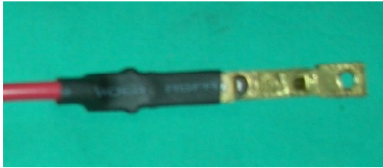
Bus Bars with leads attached
