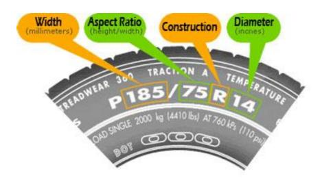
**WIDTH** - This is the width of the tire measured in millimeters from sidewall to sidewall. An example might be 215 representing 215 millimeters.
