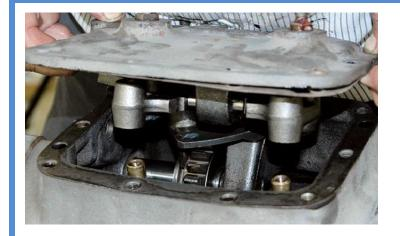
The only thing left to do is to install the side cover and reverse detent assembly
