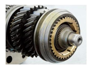
The 3 – 4 slider slips in next. The main and input shafts are now ready to be installed into the case.
