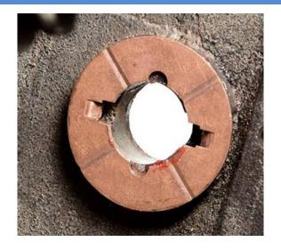
Here is a tip that will save you some frustration. As soon as you are finished cleaning the case, glue the cluster gear thrust bearing to the inside of the case with some adhesive – type silicone
