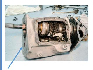
First, knock the countershaft out from the front of the case to the back. When you do, the cluster gear will drop down enough to disengage from the main shaft gears so you can pull the whole assembly out the tail shaft end of the housing. This shot shows you the main-tocluster shaft relationship. Notice there are thrust washers on both ends if the cluster. Make sure that you recover them
