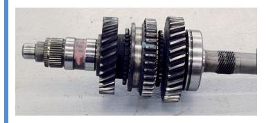
OK, now you are ready for main shaft assembly. It is just the reverse of disassembly. Before you start sliding all the parts back onto the shaft, be sure to smear high-temp grease on each of the machines surfaces that the gears / sliders ride on.
