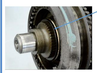
The input shaft, which is also 4<sup>th</sup> gear, simply slides of the end of the main shaft. The roller bearings inside the input shaft ride on the very end of the main shaft. Remove the snap ring slide the 3 -4 slider and 3rg gear off the front of the shaft. The rest of the gears slide off the back of the shaft.
