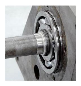
The input shaft has just one set of rollers. Grease them in place the same as the others, and the tap the input shaft partway into the case. You may need a little extra room to line up the main shaft. Once the main shaft is in place, you can install the snap ring and tap it all the way on.
