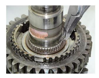
Just one more snap ring and you can pull the 1 – 2 slider and 2<sup>nd</sup> gear off the shaft. The straight cut gear attached to the 1 – 2 slider is for reverse. The main shaft in these transmissions seldom need replacing, but still check each bearing surface for any damage.
