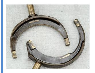
One thing to take note of is the shift forks as they are not the same, so do not get them mixed up. The bottom one is for 1<sup>st</sup> – 2<sup>nd</sup> gear slider, and the top is for the 3<sup>rd</sup> – 4<sup>th</sup>. Check for excessive wear l\on the contact surfaces, but unless they have been abused, these rarely need to be replaced.
