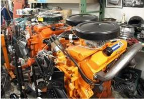
While Mosher's is best known for big orange engines with cross ram induction, this pair of single-quad big blocks shows a soft spot for the street side. The one on the hoist is a mildly hopped 383 that's headed for a '66 Coronet two-door post, the 413 on the engine stand is destined for a '62 Dart. Its Edelbrock Performer aluminum heads, Performer 440 intake and Milodon oil pan hide under a coat of correct turquoise paint. Subtlety is a key ingredient with every Mosher creation.
