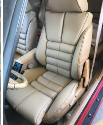
Finally got the enthusiasts driver and passenger seat installed in the Daytona Shelby Z. They are the original Dodge Daytona design with leather on top surfaces and vinyl on seat backs. Lots of sewing and cutting of all the leather pieces. The seats were recovered by Shun at N-sydez-Out in Garland, Texas. Shun did a great job sewing the complicated leather seats to the original Dodge enthusiasts' seat design.
